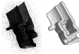
Figure 1: On the left, a point cloud sampled on a mechanical part to which 10% of outliers have been added- the outliers are uniformly distributed in a box enclosing the original point cloud. On the right, the reconstruction of an isosurface of the distance function  $d_{\mu_C, m_0}$  to the uniform probability measure on this point cloud.
